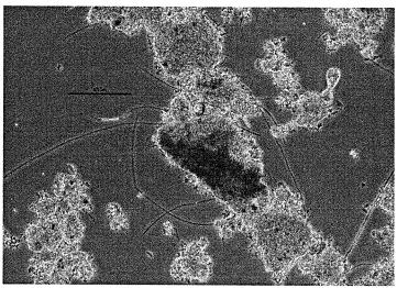
Figure 8, 100x (m), phase contrast: Floc in the AT4-2 sample appeared to be relatively dense based on brown color under phase contrast. This typically indicates good floc forming qualities. Some darker areas in floc indicated the presence of septic compounds.
