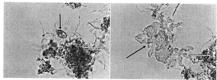
**Figure 3-400x (m):** Moderate levels of crawling ciliates (arrow) were observed. Crawling ciliates help to condense the floc by eating loosely attached bacteria around the floc edges. They are indicators of a healthy sludge age.
