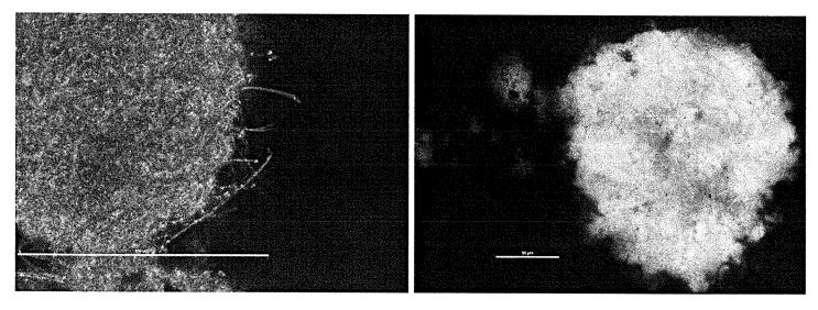
Figure 3, 400x (m), Phase contrast: Floc appeared to be tan to light brown in color under phase contrast, indicating floc high enough for good floc formation, and adequate (EPS) in the AT2-2 sample. EPS levels appeared adequate oxygen penetration throughout floc.
