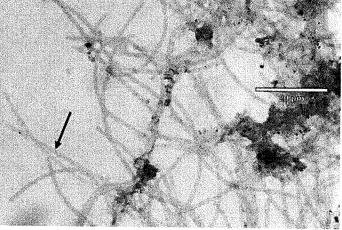
**Figure 10-1000x (m) Neisser Stain:** High levels of *Nostocoida limicola* were observed. *N. limicola* is usually associated with high levels of volatile acids in a wastewater system. *N. limicola* may also be associated with nutrient deficiency. When abundant enough, these filaments have been known to cause bulking and create a thin scum layer.
