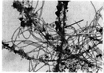
**Figure 11-1000x (m) Gram Stain:** Moderate levels of Type 0041/0675 were observed in the MLSS sample. Type 0041/0675 thrives in low F:M conditions.
