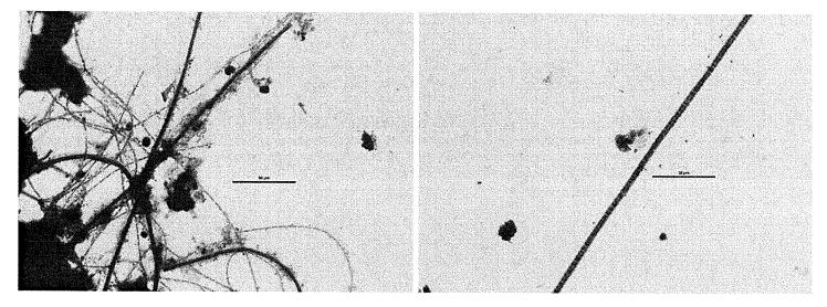
Figure 11, 1000x (m), Gram stain: Moderate levels of Type Figure 12, 1000x (m), Gram stain: *Thiothrix/*Type 021N were 0041/0675 were observed after Gram staining as well as levels of Type 1851. Both filaments tend to thrive in many Gram-positive granules. low F:M conditions.
