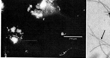
Figure 9-100x (m) India Ink Stain: Moderate levels of extracellular polymeric substances (EPS) were observed diffusing from floc and zoogloeal growths (red arrow). Diffused EPS tends to be a sign of stress in a wastewater system.
